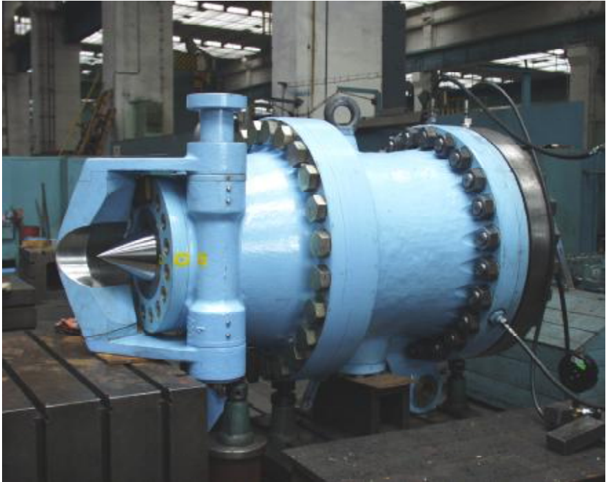
Fig. 12. Straight flow nozzle during pressure test
